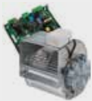
MB Brushless motor with continuous variation 0-100% of the air flow (signal 0..10 Vdc) Digital wall thermostat is an essential accessory for the operation of a unit with Brushless motor. Should not be combined with accessory TEL
